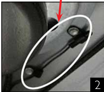
Close-up of 1/4" P-clip securing black probe.
